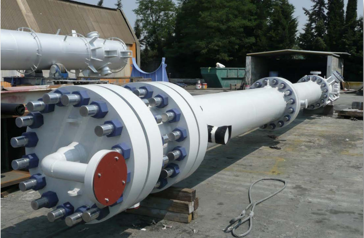
010-C-551 Purge Gas Absorber
